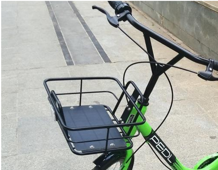
Basket has a solar panel that powers IOT lock
